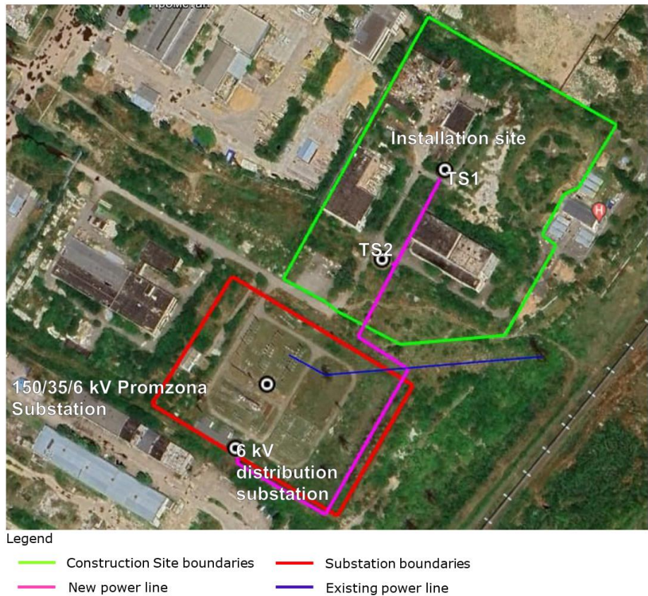
Figure 5-10: Schematic of the proposed grid connection for SPP-3
