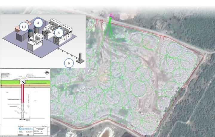
LFG simulations combined with degasification tests executed on landfill indicate that gas extracted from Melitopol landfill can power 600 kW CHP unit. Annual electricity production would be close to 600 MW. Additionally, a same amount of heat can be produced for heating purposes.
