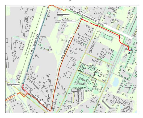
Construction of the new collector was complicated and time consuming. In the course of the construction works, it was necessary to change the layout and relocate the existing water supply lines and engineering networks, which complicated and increased the scope
