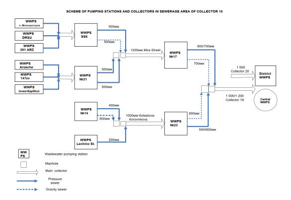
In accordance with the General Plan of Veliky Novgorod, the volume of wastewater transported through collector no. 18 will increase by 600 - 700 m<sup>3</sup>/h reaching the average flow of 2 400 - 3 100 m<sup>3</sup>/h. From this background, the existing capacity of the collector no. 18 is insufficient for the future needs.
