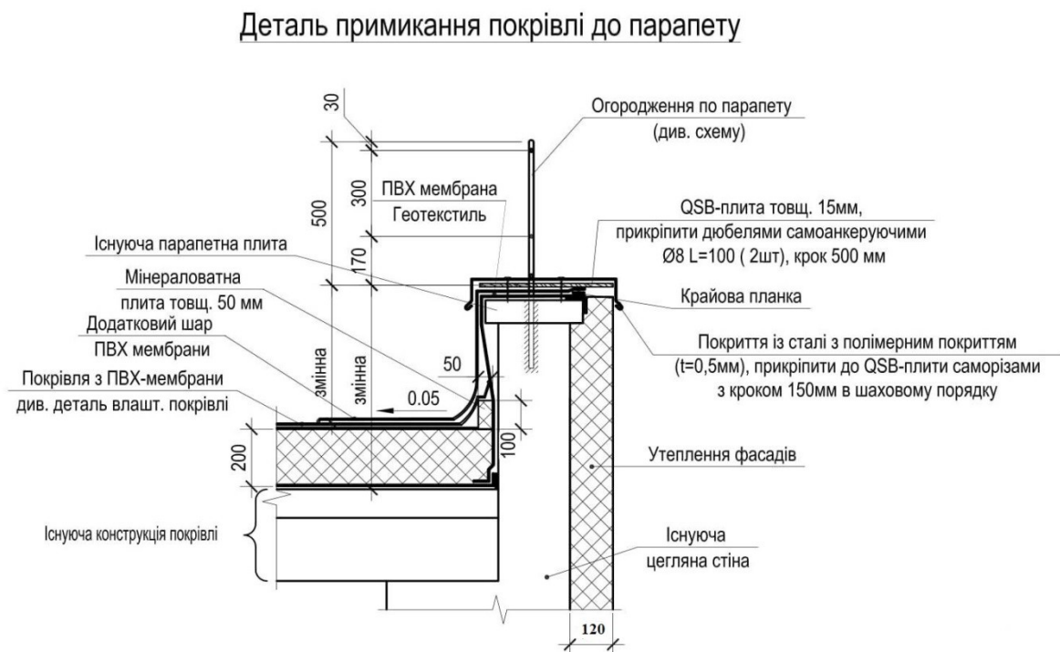
Fig. 3-5. Schemes for fastening the parapet of the roof
